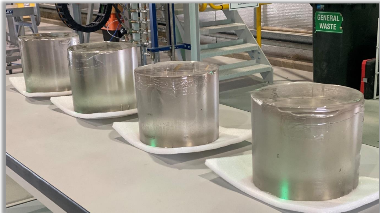
Successful sapphire boule growth from Phase A sapphire growth units
