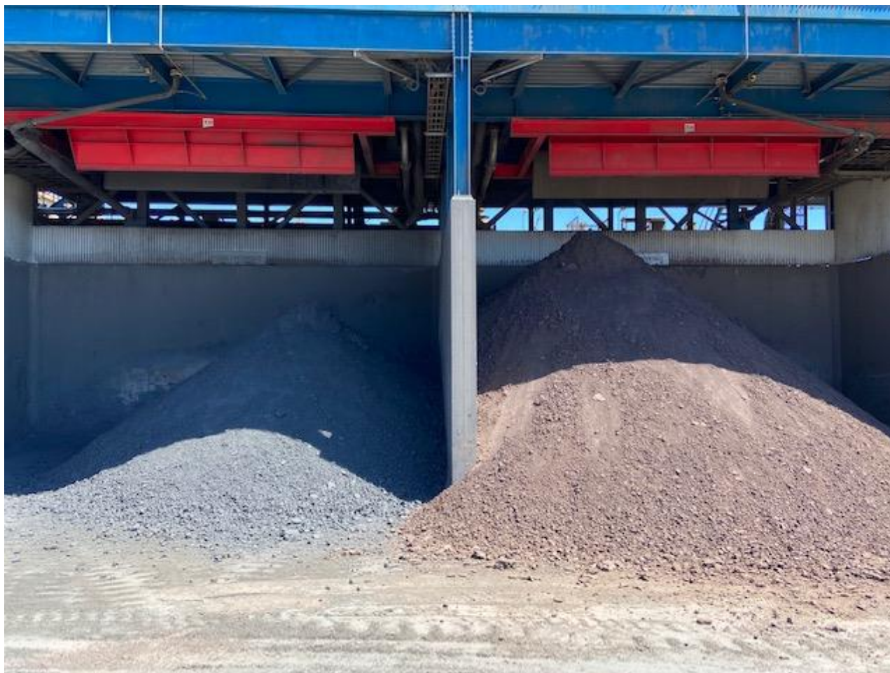
Figure 3: Filtered Federation lead concentrate (left) and zinc concentrate (right) at Peak
