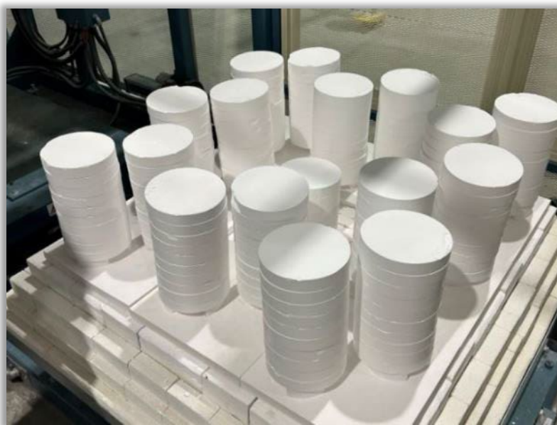
A production batch of densified, sintered HPA disc tablets (each tablet \sim 850\text{g} with density of >3.5\text{g/cm}^3 )
