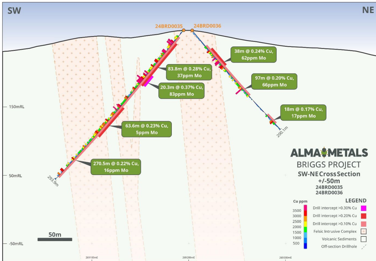
Figure 2. Cross-Section showing hole 24BRD0035 and 24BRD0036, testing the Southern Porphyry Target. For location of cross-section, refer to Figure 6.
