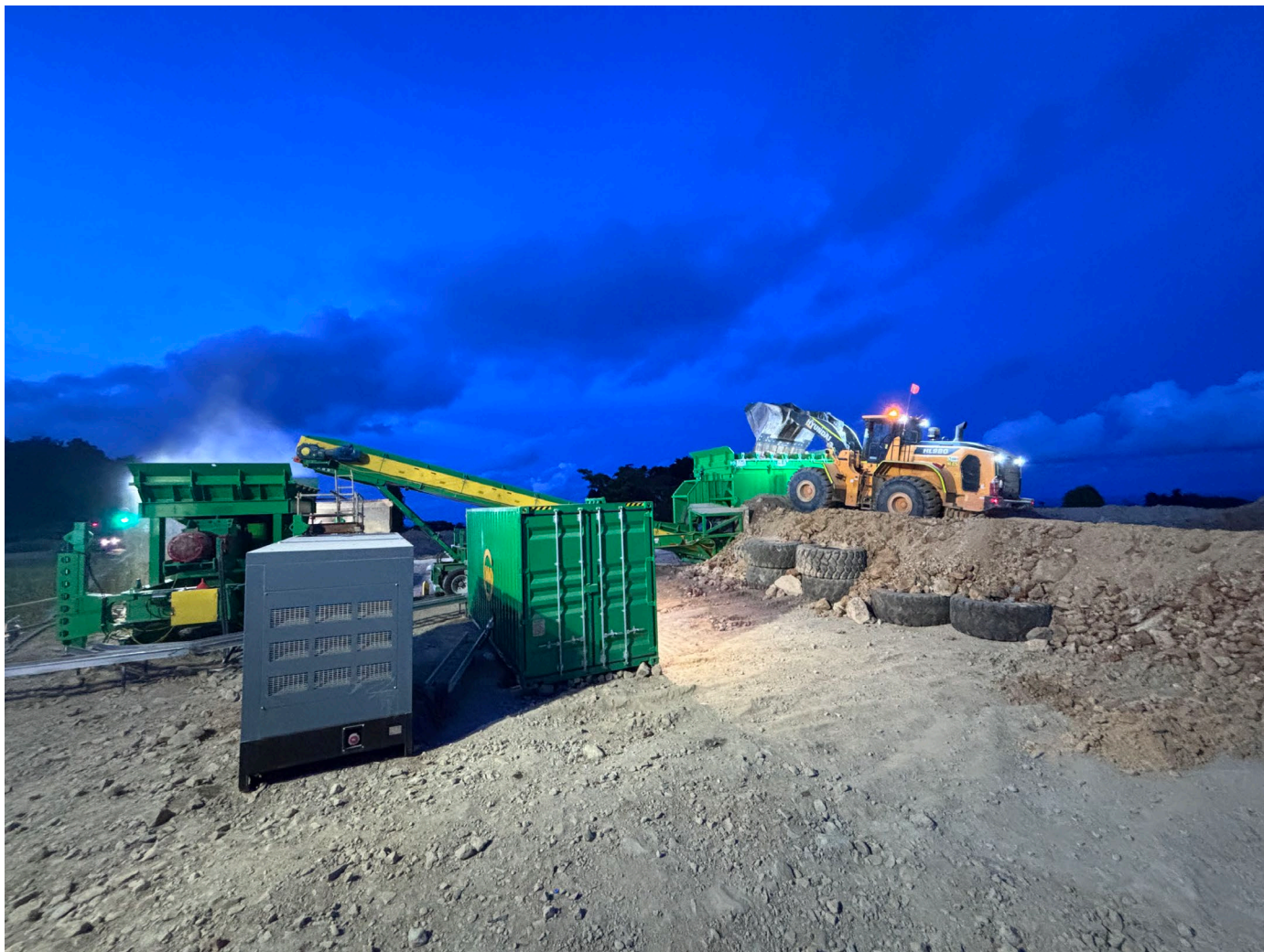
Figure 2. MMD Sizer Commissioning at Sorowar ROM Pad
