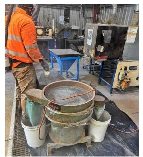
Figure 3: Screening of crushed material
