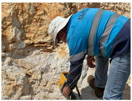
**Figure 12**. REE Target - pXRF sampling of white weathered kaolinitic fine-grained sediments adjacent to the prominent scarp as shown in Figure 12
