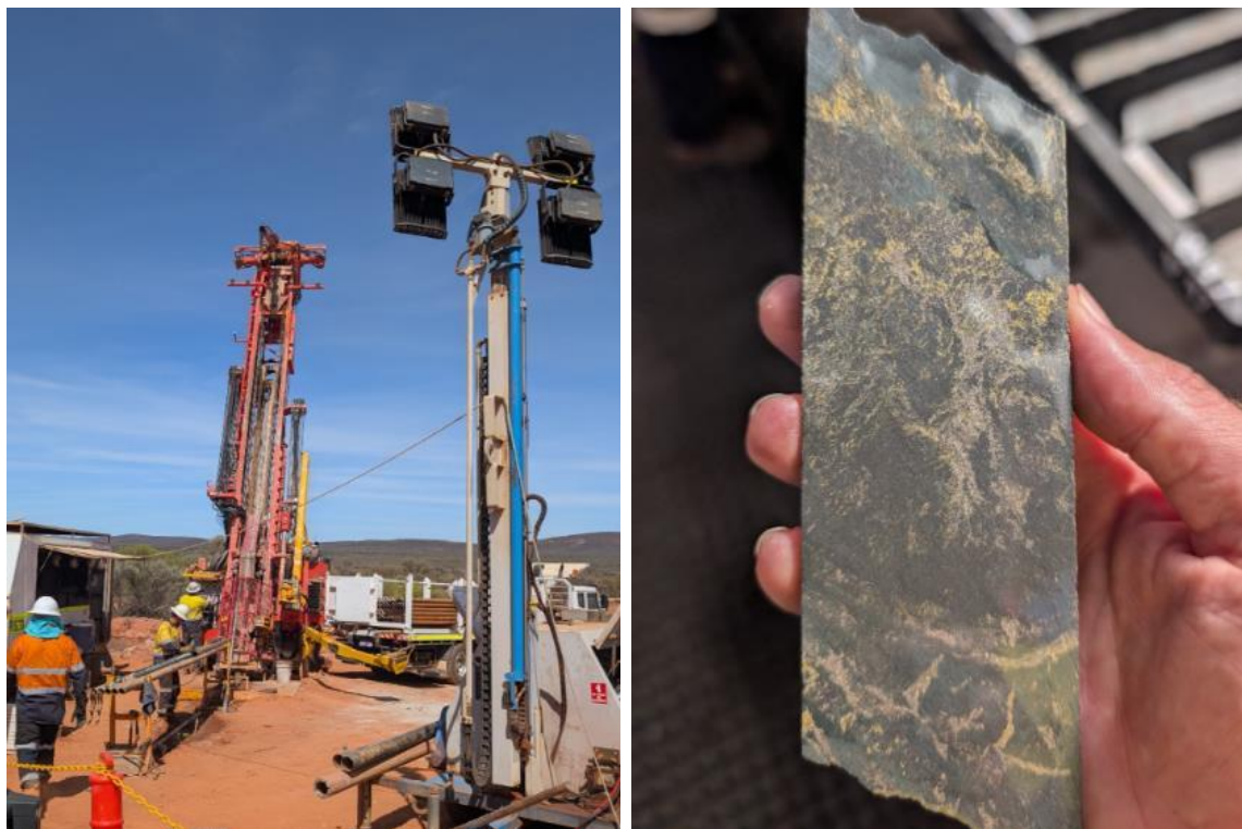
Figure 5: Grade control drilling at Gossan Valley (left). Drill core from grade control drilling at Gossan Valley (Right)
