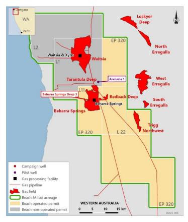
follows exploration success at Redback Deep and tested the potential of the northern extension of the Redback Terrace. Arenaria 1 intersected gas in the Kingia reservoir however wireline logs indicated poor reservoir quality. The well was subsequently plugged and abandoned.
