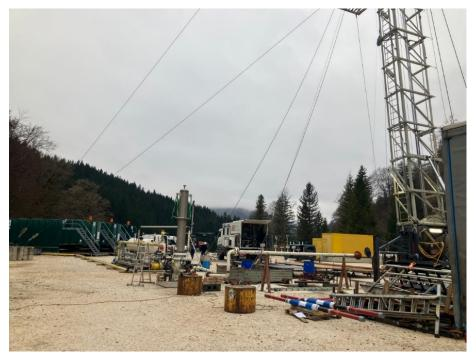
Well completion operations and Flow Testing Facilities set up at the Welchau-1 well location
