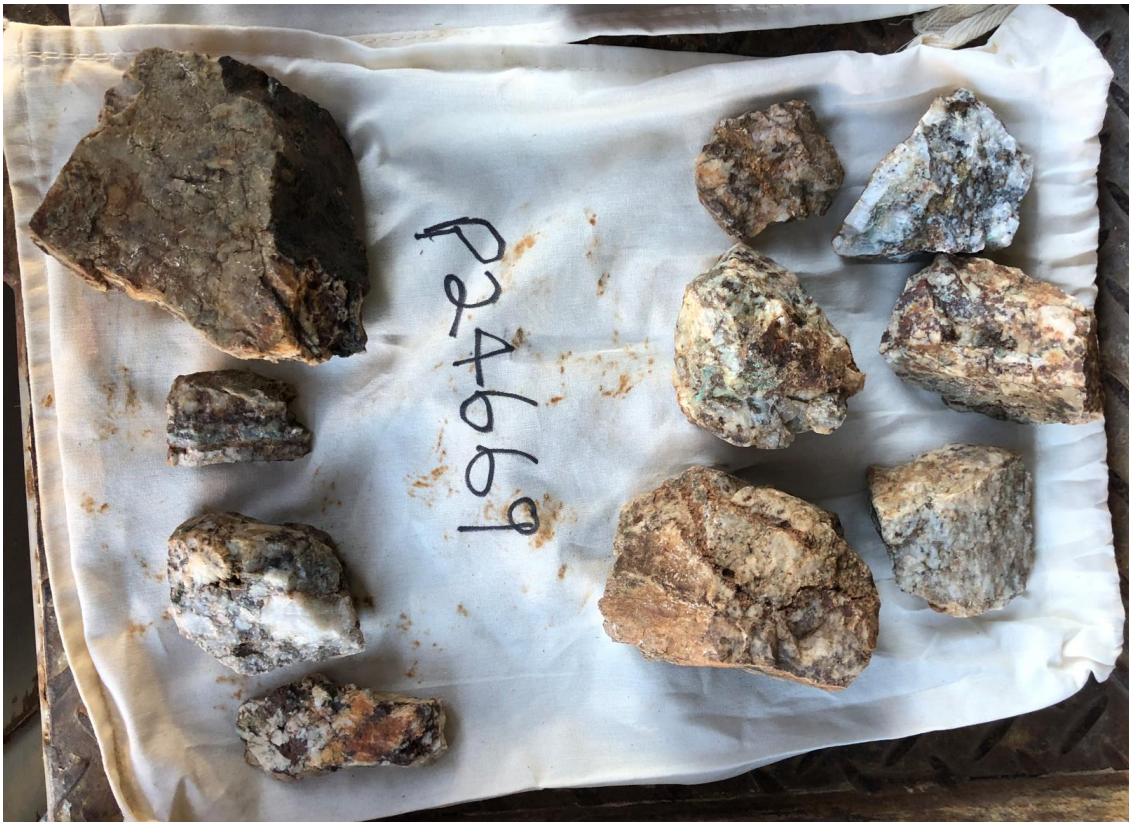
Figure 2: Sample P24669 grading 10.65 g/t Au, 1.98% Cu & 158g/t Ag
