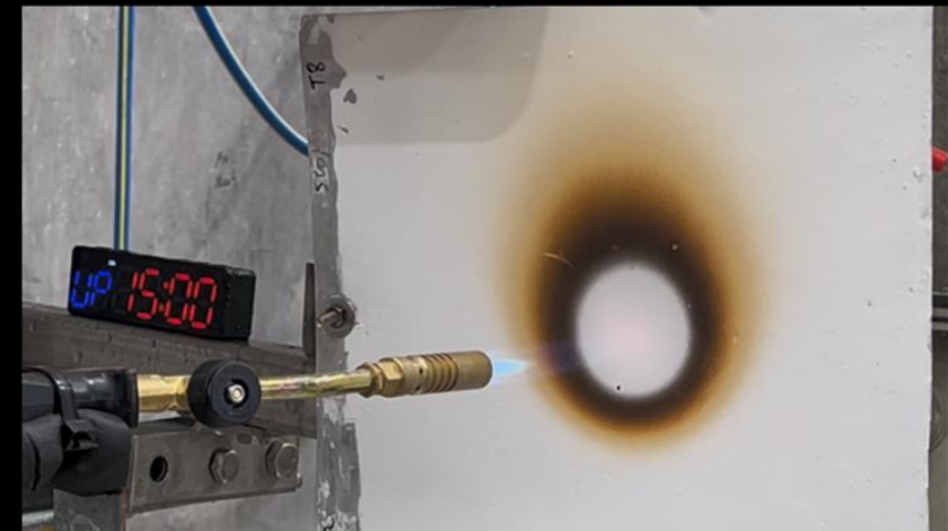
ULTRACOATED (0.3MM) ALUMINIUM CELL CASE Cell case integrity intact after 15 minutes burn test
