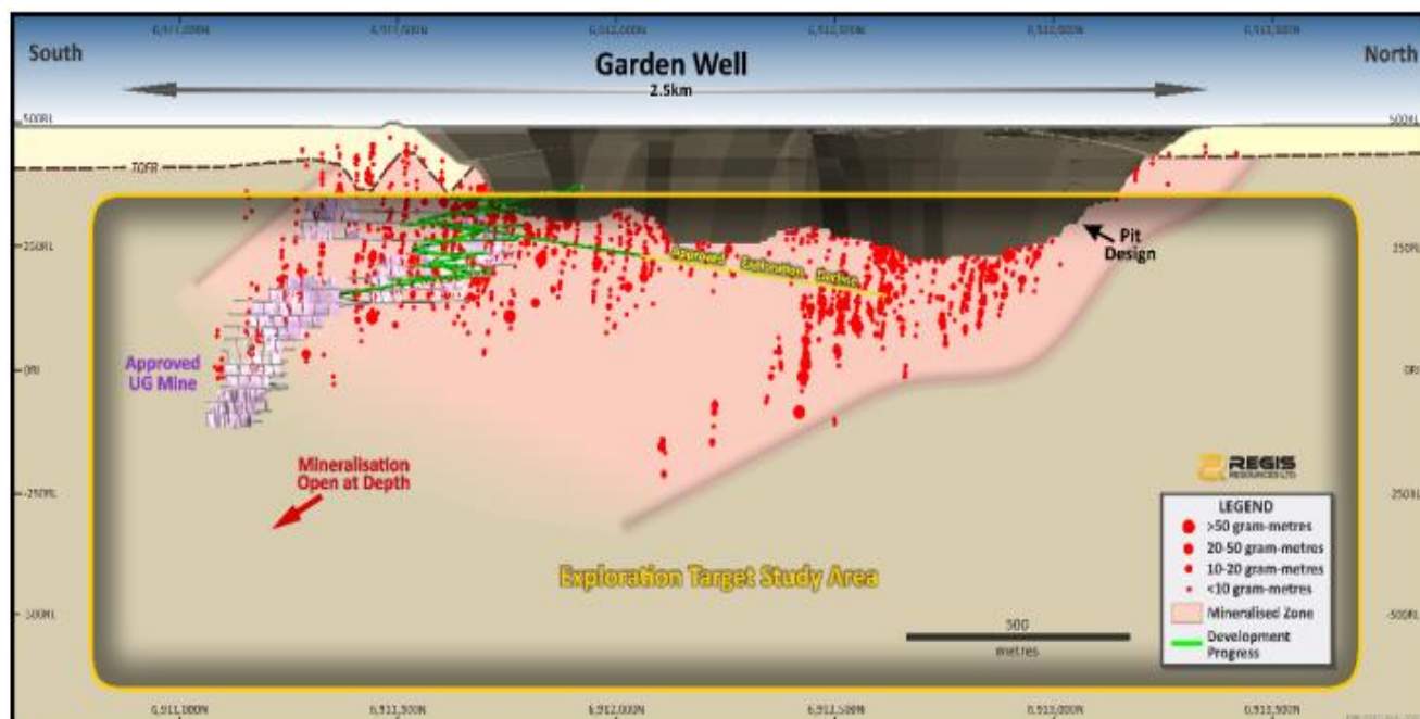
Figure 6: Original Garden Well long section looking west showing the Exploration Target Area at the time expenditure to explore the area to the North was approved.
