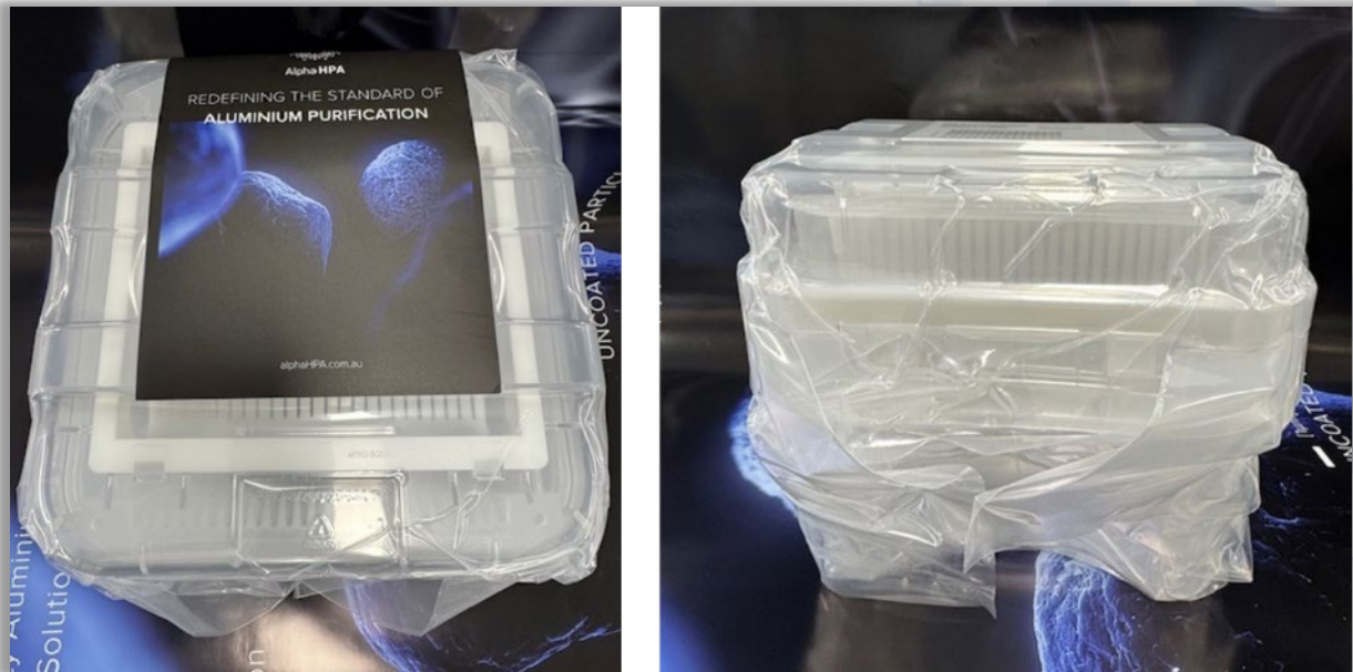
Cassette of completed 8" (200mm) sapphire wafers for GaN-on-sapphire semiconductor end-user (RHS)
