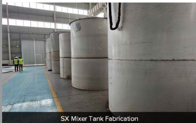
Selected images showing offsite fabrication of Solvent Extraction (SX) Modules
