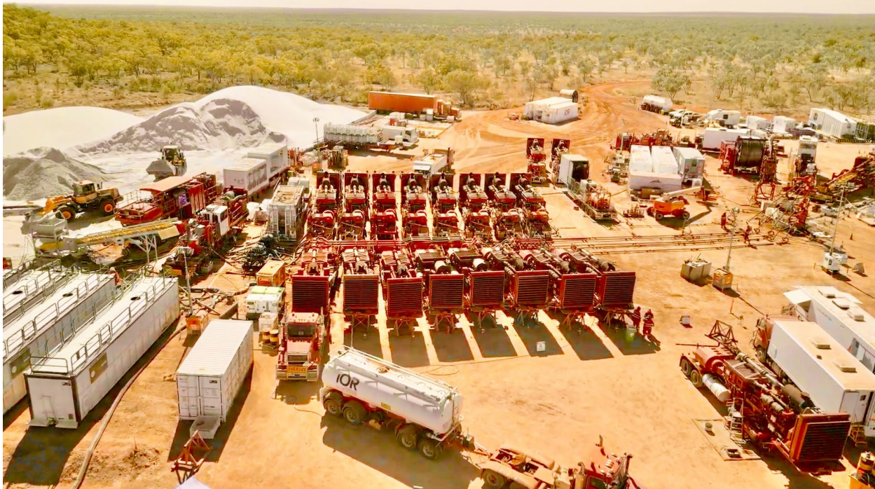
Hydraulic stimulation pump equipment being set up at the Carpentaria-5H well pad
