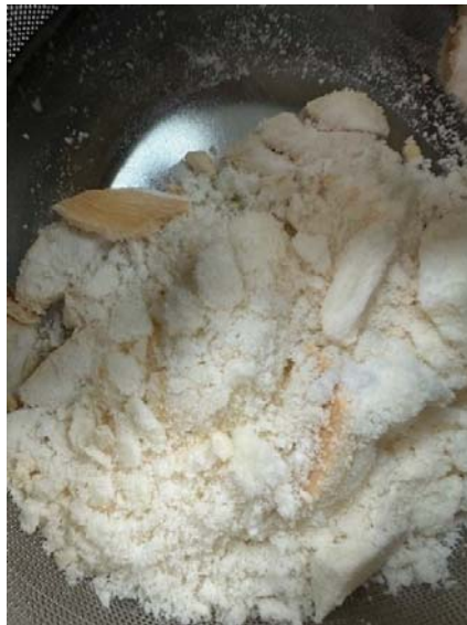
Figure 10.4: Boric acid crystals after continuous crystallization test (CRZ1-4) and centrifugation
