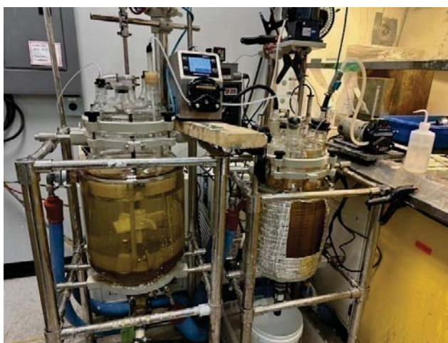
Figure 10.2: Boric acid continuous crystallization set-up including an agitated feed tank
