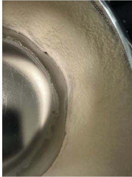
Figure 10.4: Boric acid crystals after continuous crystallization test (CRZ1-4) and centrifugation
