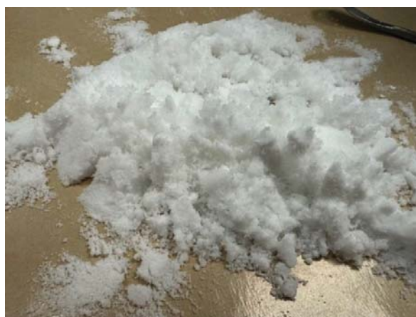
Figure 10.6: Boric acid crystals after re-crystallization and dewatering process
