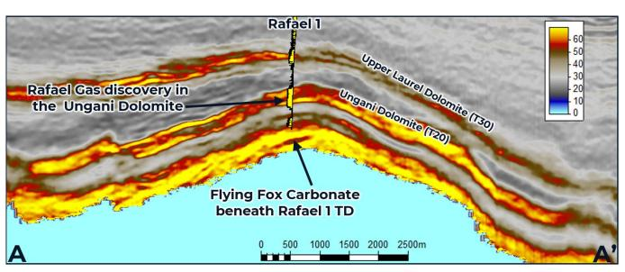
Seismic inversion - a method to determine carbonate reservoir presence
