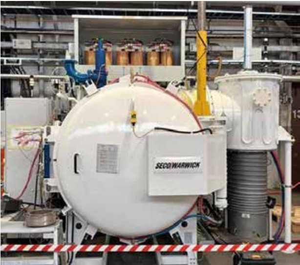
Vacuum braze furnace during factory acceptance testing to 1,200 °C and 5x10 -5 mbar
