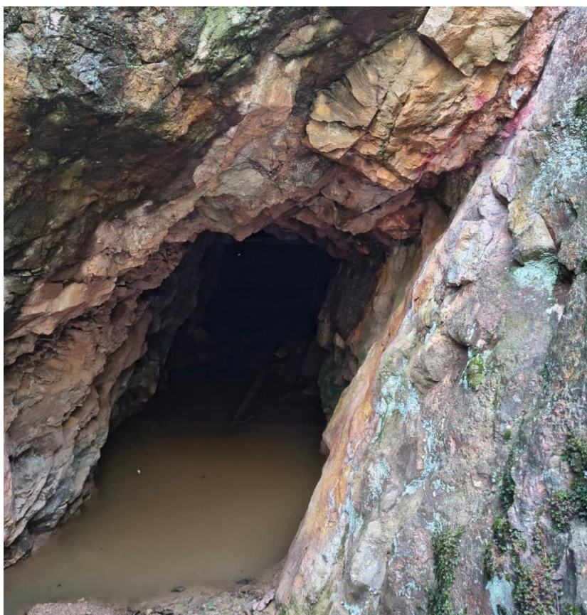
Figure 1. Previously unmapped colloform quartz veining associated with a small historic adit. Assays of the vein (upper right corner) returned 30g/t Ag & 20.4g/t Au (1,594g/t AgEq 1 , sample 825486) .
