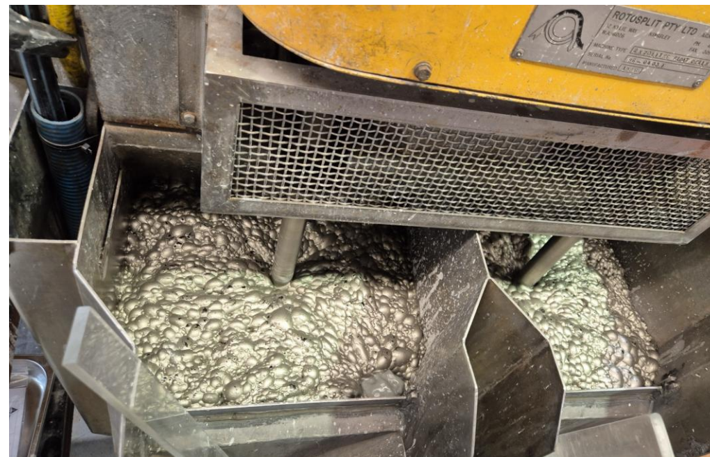
Rougher flotation – 98.3% sulphur recovered concentrate, 91.6% of the gold
