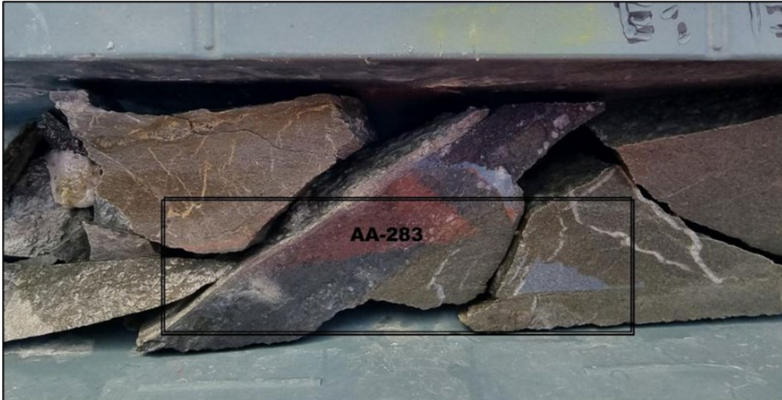
Core tray photo of AA-283 (CND03, ~177.85m) showing Sb-bearing veining (stibnite)
