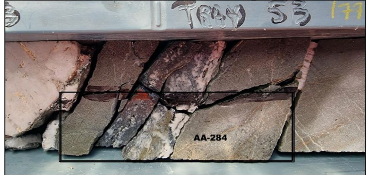
Core tray photo of AA-284 (CND03, ~177.46m) highlighting Sb-mineralised structures
