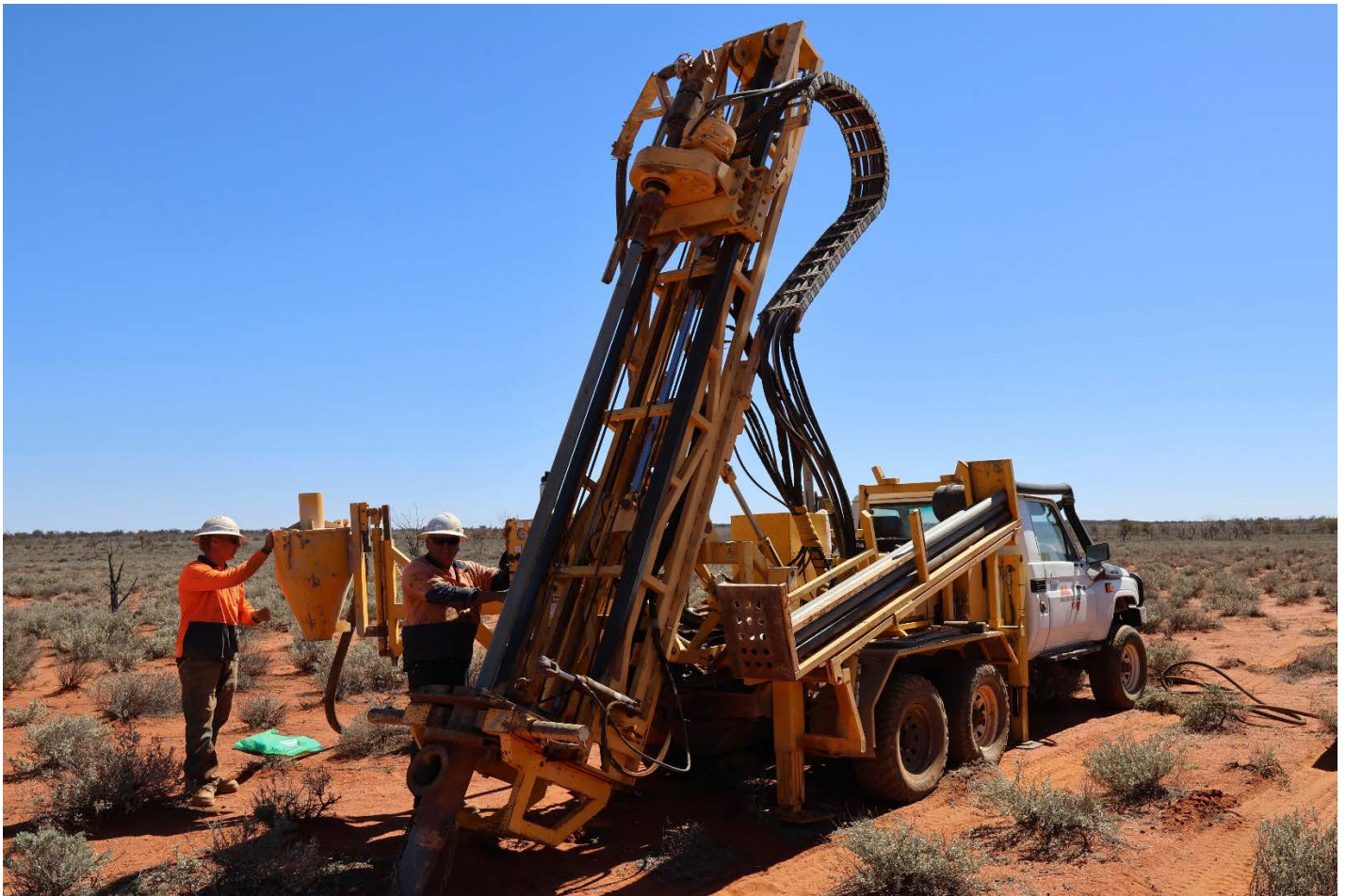
Figure 3: Landcruiser mounted AC Drilling underway at Ariadne-Company Well prospect areas, Minos Gold Project.
