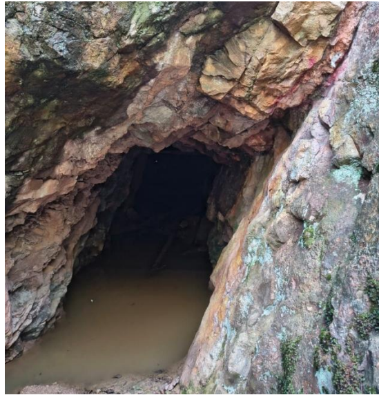
Figure 8. Previously unmapped colloform quartz veining associated with a small historic adit. Assays of the vein (upper right corner) returned 30g/t Ag & 20.4g/t Au (1,594g/t AgEq) 4,5 .
