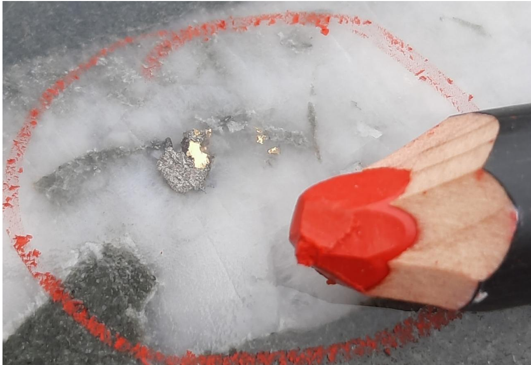
Figure 14. Visible gold* grains (lustrous yellow) up to 2mm associated with sulphides (grey) in quartz from AMD014A at 465.0m 11 . Assays are currently pending for this hole.
