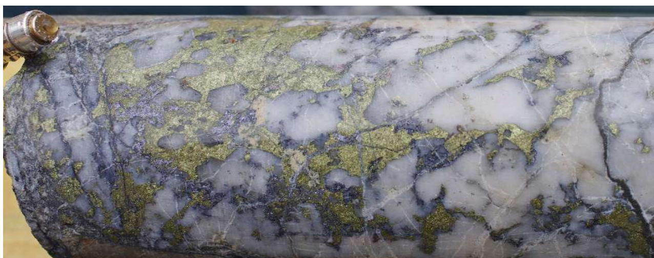
Figure 3. Strongly mineralised magmatic quartz vein at 118.4m depth in hole 24BRD0036, NE side of Southern Porphyry, containing intense chalcopyrite-molybdenite mineralisation. Within a 2m sample which assayed 0.81% Cu and 701ppm Mo. Core diameter 61.1mm.
