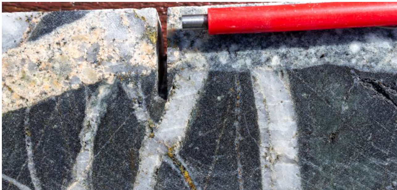
Figure 4. Mineralised volcaniclastic sediments at 347.7m depth in hole BD019003, Briggs Central. Within a 1m interval which assayed 0.49% Cu and 9ppm Mo. Note porphyry style B-veins containing quartz-chalcopyrite-pyrite in volcaniclastic sediment are cut by later granite porphyry dyke.
