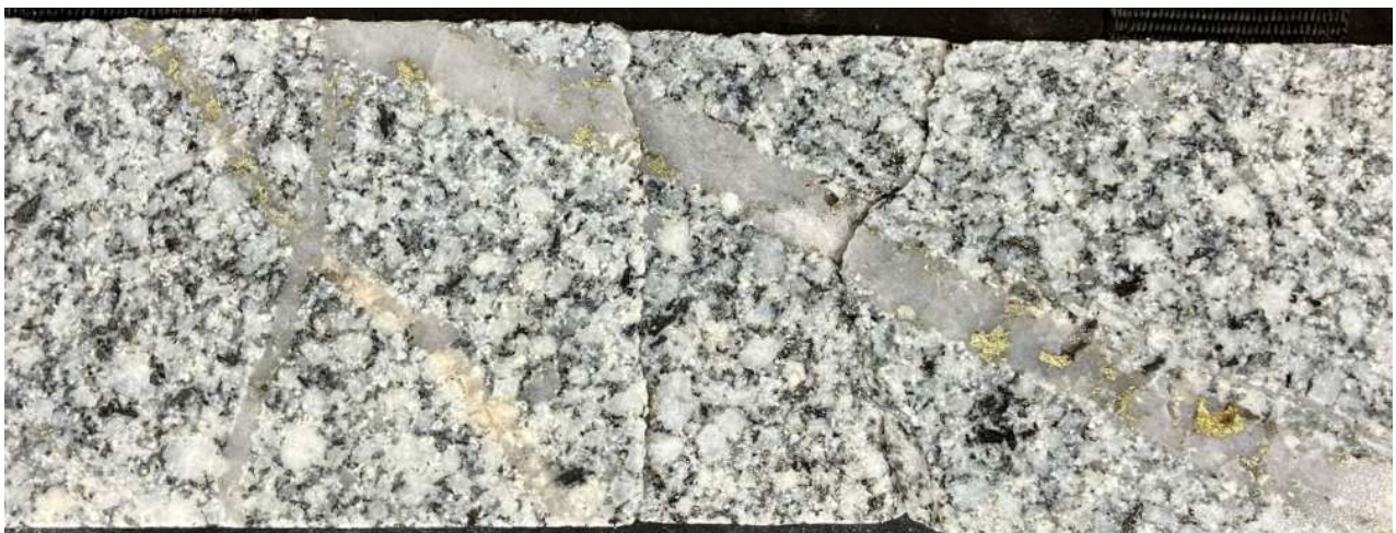
Figure 2. Copper sulphides in quartz-vein stockworks hosted in potassic altered porphyritic granodiorite , Briggs Central. Hole 23BRD0016 at 123.5m. Within a 2m interval of 61mm diameter core which assayed 0.31% Cu.
