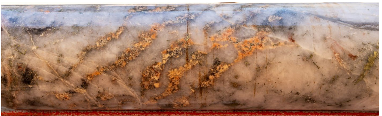
Figure 5. UST textured magmatic quartz body at 495.7m downhole depth in 25BRD0037. From within a 0.6m wide interval visually estimated to contain 1% chalcopyrite (0.35% Cu*). Core diameter 61mm.
