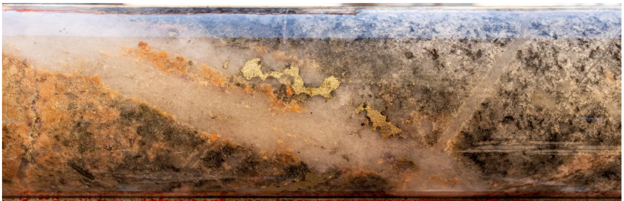
Figure 4. Composite B-vein with quartz and chalcopyrite in altered granodiorite porphyry at 525.5m downhole depth in 25BRD0037. From within a 17.4m wide interval visually estimated to contain 0.75% chalcopyrite (0.25% Cu*). Core diameter 61mm.
