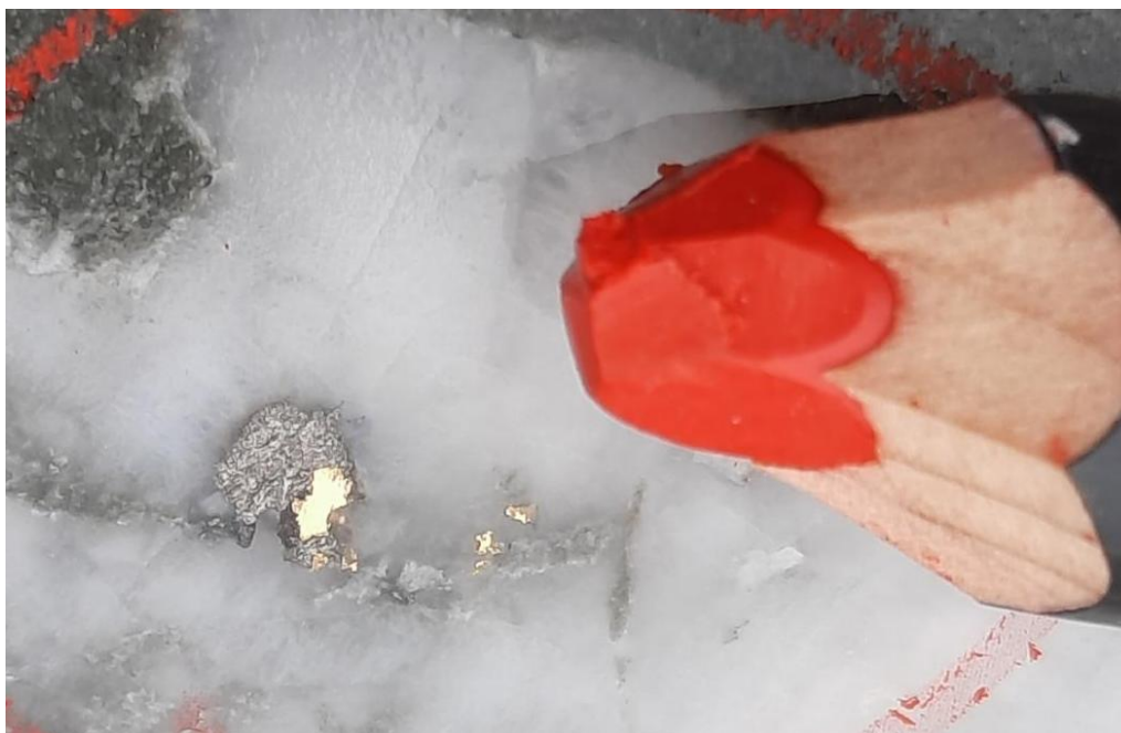
Figure 2. Visible gold grains (lustrous yellow) up to 2mm associated with sulphides (grey) in quartz from AMD014A at 465.0m 1 . Assays are currently pending for this hole. Note: In relation to the disclosure of visible mineralisation, the Company cautions that visual estimates of mineral abundance should never be considered a proxy or substitute for laboratory analysis. Laboratory assay results are required to determine actual widths and grade of the visible mineralisation reported in preliminary geological logging.
