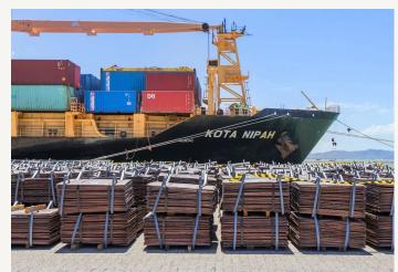
Eloise copper concentrate is trucked to Mt Isa, where it is smelted into copper anode. That anode is then railed to Townsville to be refined into 99.995% pure copper cathode.
