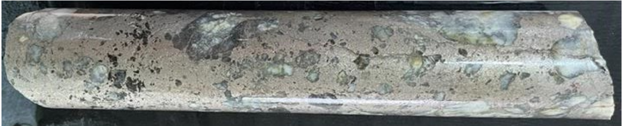
Figure 4. Core photo – massive sulphide breccia from ATDD001 at approximately 413m downhole. Dominantly pyrrhotite with minor chalcopyrite replacing quartz-carbonate. Core diameter is 50.5mm.
