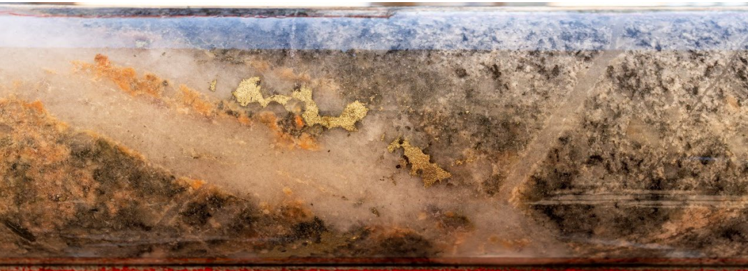
Composite B-vein with quartz and chalcopyrite in altered granodiorite porphyry at 525.5m downhole depth in 25BRD0037. From within a 17.4m wide interval visually estimated to contain 0.75% chalcopyrite (0.25% Cu*). Core diameter 61mm.
