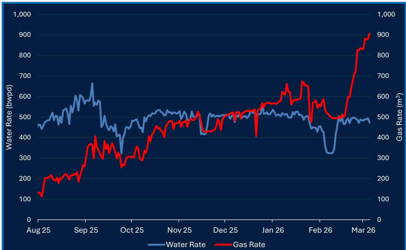
Pilot Well Project gas and water production showing 900% increase in gas rates since August 2025
