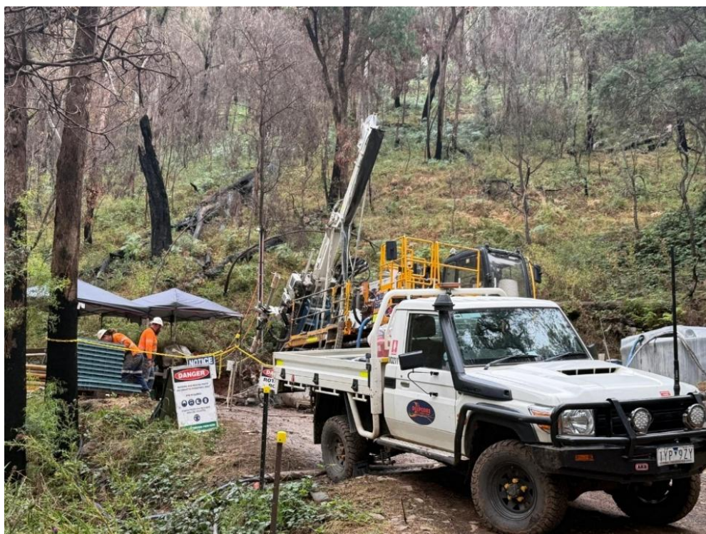
Figure 1 Photograph of the diamond rig on site at the Happy Valleys deposit, set up to complete deep hole AMD023.
