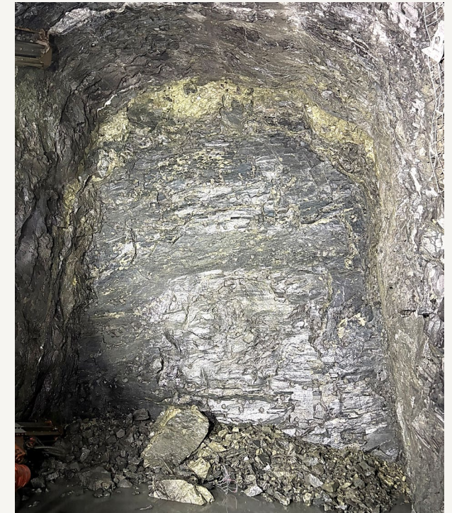
Development face passing through the J1 lens at Jericho, showing visible copper sulphide mineralisation. Face dimensions are approximately 5.5m wide by 7.5m high 1,2 .
