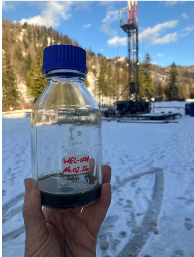
Figure 14: Showing oil recovered from the Reifling Formation during testing
