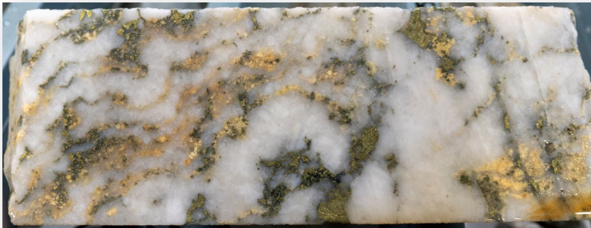
Magmatic quartz with micro-UST textures (unidirectional solidification textures) and chalcopyrite at 55m downhole depth in drill hole 25BRD0038. From within a 30m wide interval which assayed 0.9% Cu. Core diameter 61mm.
