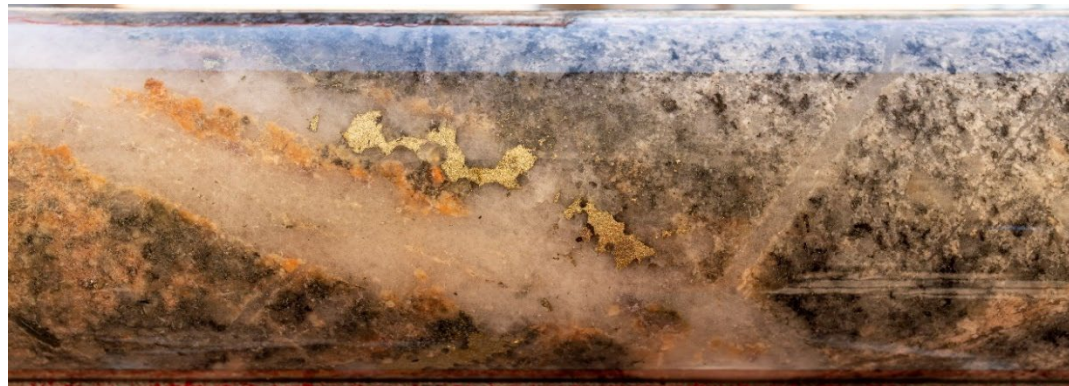
Composite B-vein with quartz and chalcopyrite in altered granodiorite porphyry at 525.5m downhole depth in 25BRD0037. From within a 2m wide interval which assayed 0.3% Cu. Core diameter 61mm.
