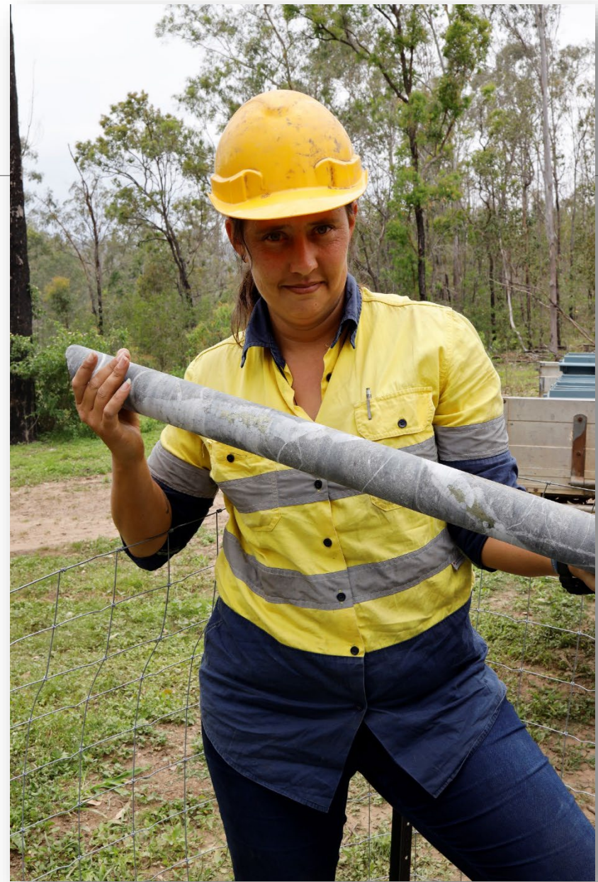
Quartz-chalcopyrite veined volcanic sediments at 169m downhole depth in drill hole 23BRD0024. From within a 2m wide interval which assayed 0.7% Cu. Core diameter 61mm.
