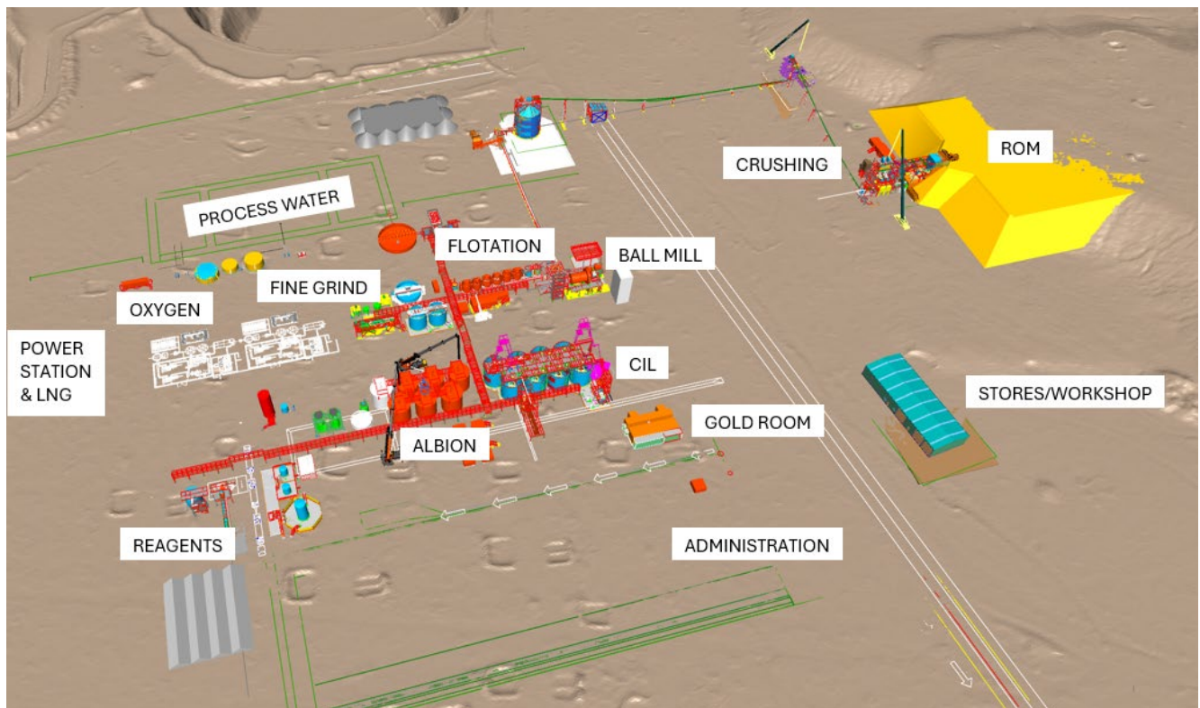
Figure 5 – Process plant working layout
