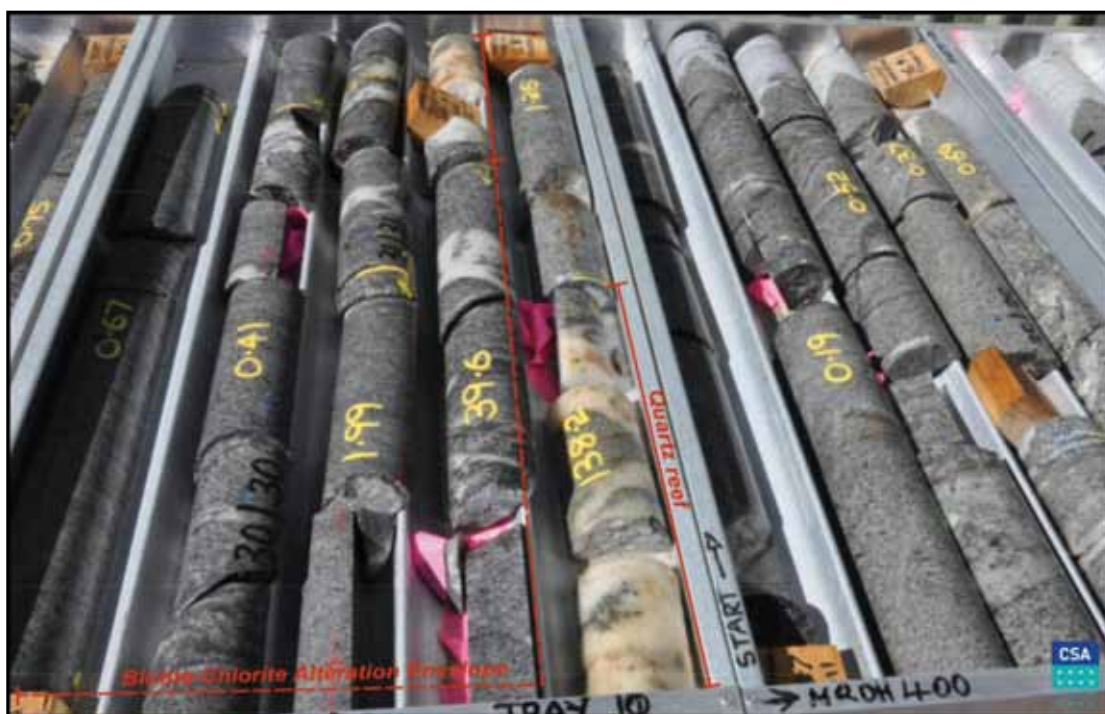
Figure 4 – Drillhole MRDH400 displaying the development of Quartz Reef in the Biotite-Chlorite Stockwork envelope, gold grades (g/t) are written in yellow on drillcore.
