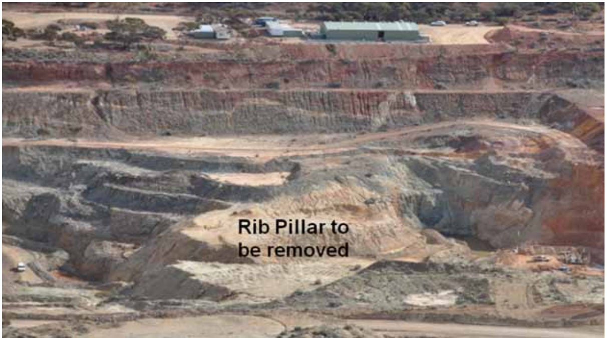
Figure 8 – Rib pillar to be removed to allow for pit floor extraction to provide constant elevation full width of tonalite and mining parcel for model reconciliation.
