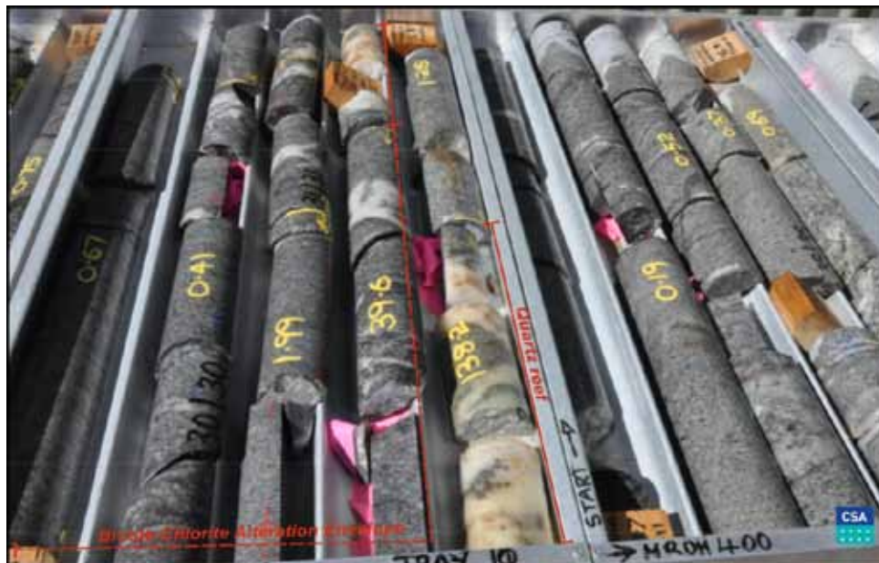
Figure 8. Drillhole MRDH400 displaying the development of Quartz Reef in the Biotite-Chlorite Stockwork envelope, gold grades (g/t) are written in yellow on drillcore.
